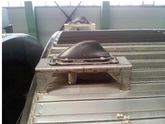
*An example of a train antenna installation*
